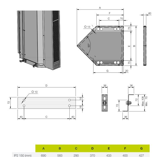
Index: The dimensions above display the installation components of the IP2. The vertically mounted unit dimensions above display the measurements of the base plate.
