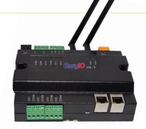
The unit retains the widely used BACnet MS/TP and Modbus protocols for more traditional installations, so you always have an option for integration especially useful when mixing manufacturers.
